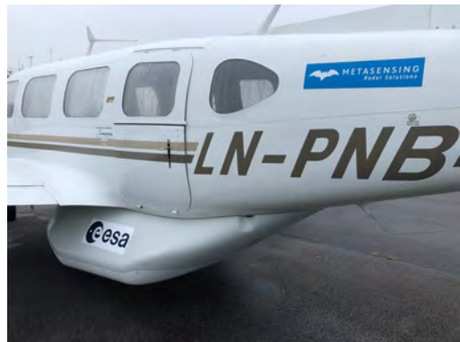
Figure 2 The aircraft and belly pod where the OSCAR system and gimbal are installed.
