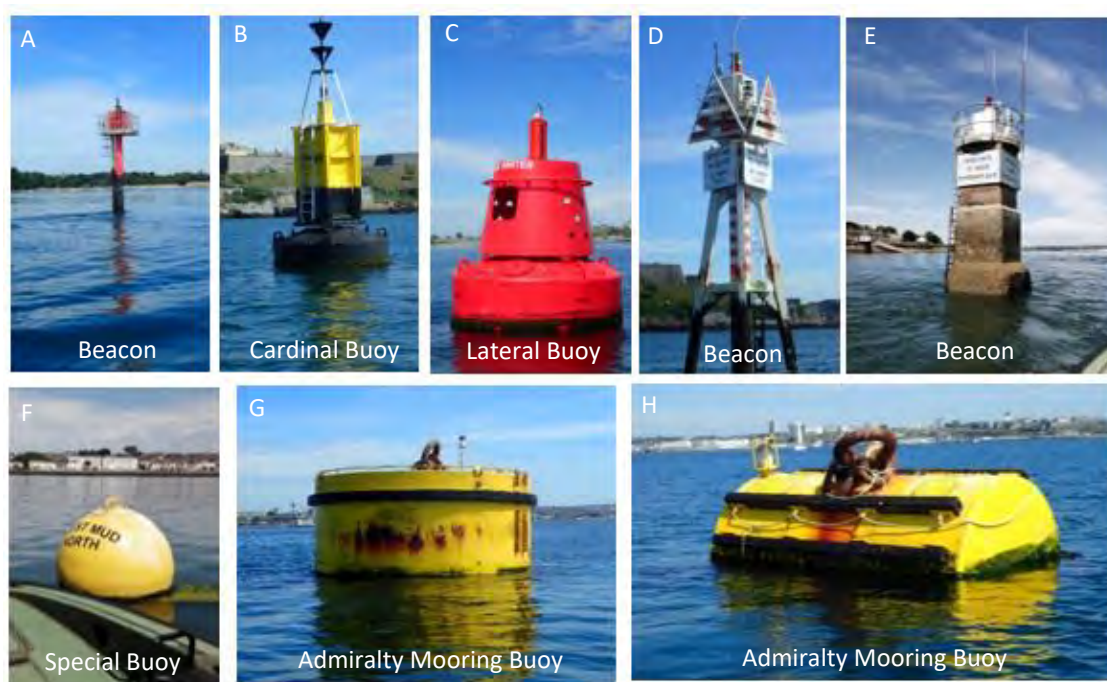
Figure 1. A – H show examples of the range of shapes, sizes and construction materials of AtoN in Plymouth Sound (Images©Sara McGourty).
