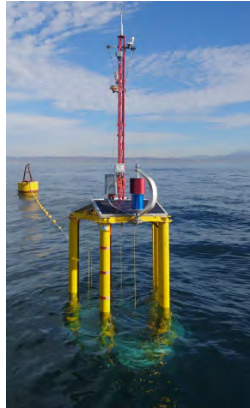
Figure 1: Instrumented buoy BOMM (Boya Oceanográfica y de Meteorología Marina) deployed in the coastal North-East Pacific.
