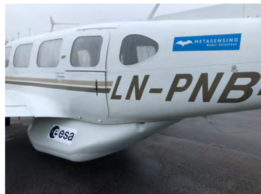
Figure 2 The aircraft and belly pod where the the OSCAR system and gimbal are installed.
