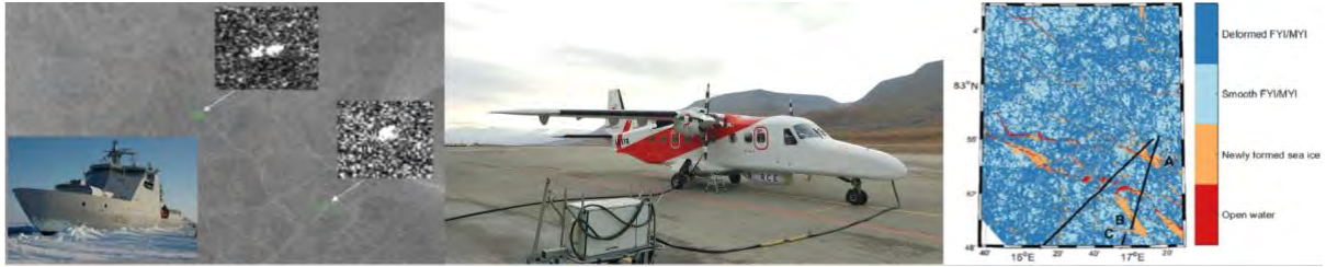
Figure 2. Left: Ship detection in ice-infested waters based on Dual-Polarization SAR (Brekke & Anfinson, 2011). Middle: Lufttransport's Dornier DO-228 aircraft (LN-LYR). Right: Sea ice identification and categorization based on SAR satellite images (Johansson et al., 2017).
