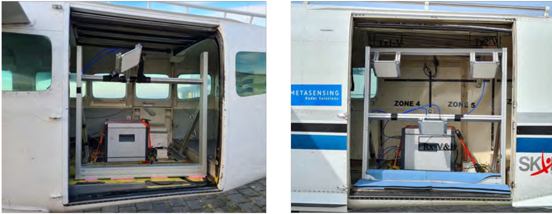
Figure 1: Left: bistatic receive-only radar installed on the leading aircraft, with the dual-pol antenna tilted to provide overlapping antenna footprints. Right: transmit-receive system installed on trailing aircraft, with two transmit antennas toggled in order to implement ATI.
